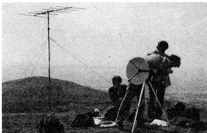
Setting frequency on 10GHz. The 144MHz talk-back antenna is located close to the 10GHz equipment, enabling both sets of gear to be operated simultaneously. When not operating full duplex, this will considerably speed-up operation and it will also allow the received signal to be retransmitted via talk-back, permitting easy optimization of the (distant) dish
