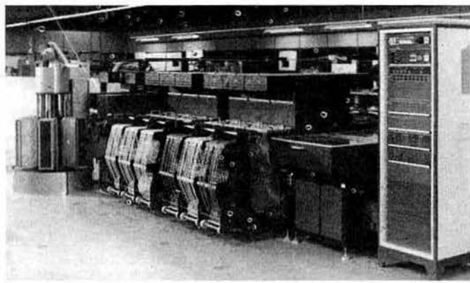
Photo 3. A far cry from the kitchen table! A modern, multi-head automatic placement machine. Typically with eight placement heads, each mounting 25 components, some 200,000 components are put on to 1,000 boards in an hour. Despite the need for specialized servicing and virtual impossibility of d-i-y modifications, this—for better or worse—is the way the electronics industry is going. (Mullard Ltd)
